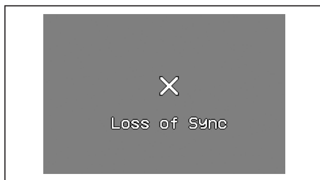
Figure 3. CVBSOUT in Demo Mode During LOS (NTSC)
